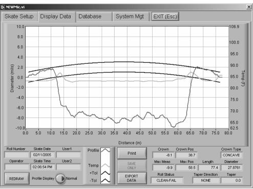
Figure 3: Dirty Skate Graphic Display Showing: Tolerance Bands at +/- 0.001" Thermal Profile at 83<sup>0</sup> F to 87<sup>0</sup> F Physical Profile with 0.010" Wear Pattern
